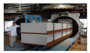
2.9 m Diameter X 44 m Long X 4 Nos Autoclaves.
