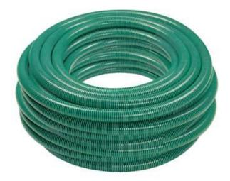
The hose shall consist of a flexible thermoplastics material supported in its mass by a helix of thermoplastic material of similar molicular structure. The reininforcing and flexible component of the wall shall be fused and free from visible cracks, porosity, foreign inclusions or other defects such as are liable to cause failure of these hoses.
