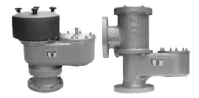
Breather Valve is a low pressure & vacuum relief valve enclosed in one housing. These are intended to use where pressure and Vacuum relief is required. These low-pressure, high-flow Valve automatically adjust the container / storage tank pressure with respect to environmental pressure changes and prevent excessive differentials during airlifts and reduce evaporation Losses.
