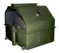
online Magnetic Separators are available for installation in the Feed lines such as at the outlet of elevator, screw conveyor etc. Flanged type Inlet and outlet connections are provided. The Magnetic Drum incorporates High Intensity strontium / Rare Earth Magnets. These are widely used for Cattle Feed Plants, Flour Mills, Rice Mill, Minerals, Refractoriness, Glass and many other Products.
