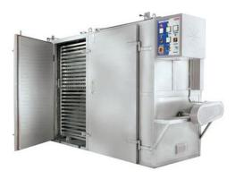
The Body of Tray Dryer is made of Mild Steel Sheet either painted or Powder coated. The trays and other contact parts are made of Aluminum / Stainless Steel depending upon product requirement and buyer choice. The dryer is equipped with fans for air circulation and heating elements. The Temp can be varied from Room Temp. to 1000 depending upon products requirement and humidity level.
