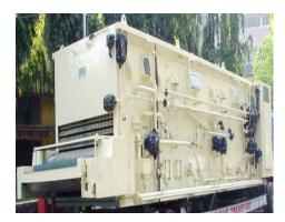
Glass bottles after recovery from the market require a through and consistent cleaning with detergent and heated water. To fulfill this purpose and ensure highest level of cleaning we supply a Single or Multi Soak bottle washer based on plant capacity and the clients need.
