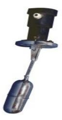
Hermitically sealed reed switches are enclosed inside the sensor stem, which are actuated by the magnetic floats. Being compact in size these are used in small tanks and equipment. These are specially designed to encapsulate permanent magnets inside them. These also traverse up / down or tilt outside or on one side of the sensor stem.
