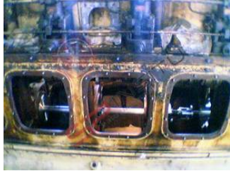
INSITU Line-Boring of Main Housing of SKL 1100KVA Diesel Engine
