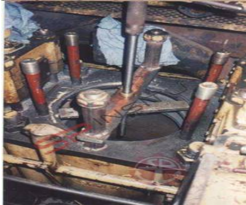
The METAL-STITCHED areas are being machined finally to facilitate perfect seating of Liner Collar
