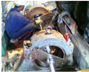
INSITU Boring-Vertical Raw Mill Rocker Arm co-axial Housing in a Cement Industry
