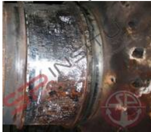
RawMill Trunnion Journal (FLSmidth Make-Dia 1300mm) in a Thermal Power Plant -Before INSITU Grinding
