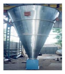
Conical Screw mixer/blender or Vertical Screw blender or Nauta mixer is made based on the principle of rotation and revolution, conveying the material along with the axle by means of rotation.
