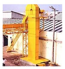
We manufacture and supply high performance bucket elevator which are used in elevating and discharging fruits and vegetables such as mangoes, apples, guavas, citrus and others from the end of one process to the next.
