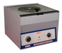
Compact model for routine work in medical and industrial laboratories. The special featur include. Easy lid lock, stepless speed regulator and timer
