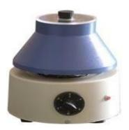
A low Priced units meeting the small capacity centrifuging reqrirements of medical practitioners, pathological laboratories requirements of medical parctitioners, pathological laboratories and hospital for routine centrifuging tests. The unit are fitted with resiliently mounted motor for vibration free performance having built is 5 step speed regulator and non-removable swing-out rotor complete with tube carriers.
