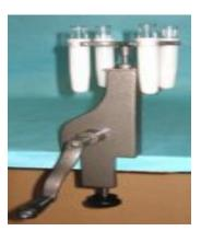
For Four Tubes. Single speed, hand driven machine consisting of a substantial cast iron body enclosing a steel pinion and worm drive fitted with a ball-thrust race. With removable crank handle and one thumb screw clamp to clamp the machine to a table. The head has captive union rings to accommodate 15 ml buckets. Body baked hammertone finish. Complete with plastic buckets and glass centrifuge tubes.
