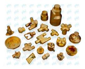
Wide range of forging enable us to forge brass from 20 Gram to 12 KG weight. All forging dies are designed in-house and other processes are outsourced.
