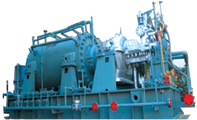
Centrifugal compressor for H2 recycle application
