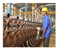
Boiler Header is a manifold which tie multiple steam carrying pipes to one boiler. The manufacturing requires precision drilling of the holes for pipes with close tolerance, fabrication and heat treatment. Boiler header are designed for 47 Kg/Cm² pressure & 364°C temperature. The Boiler Headers are usually made from Chromium-Moly Steel like P11
