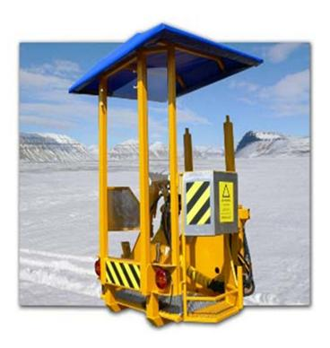
Stickset-light is a manual machine for deployment of snowsticks. A person needs to work on the machine, and drive all movements manually with handles. The stick is put in to the ground by hand.
