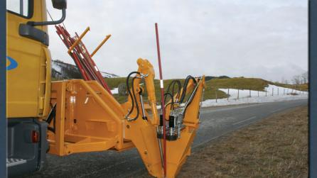
The machine controles the depth of the pole, to ensure the pole i put correctly in to the ground..
