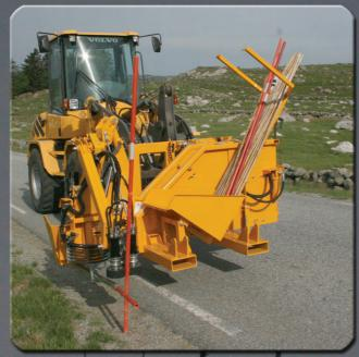
**Converting the machine for removal of snow poles are easy.**
