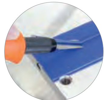
Easy removal of the welding bead with the supplied tool
