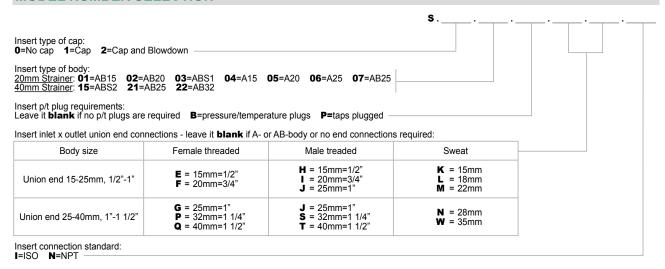
Example: S.1.01.P.I=Strainer in AB 15mm ISO female threaded body with plugs.
