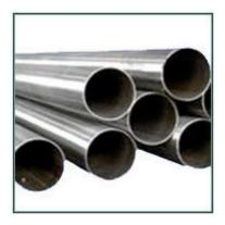
The alloy is stabilized with Columbiam to minimize carbide precipitation during welding. It has good mechanical properties and can be fabricated with comparative ease. Although the alloy was designed for use in sulfuric acid related industries, it finds wide usage throughout the chemical processing industry.
