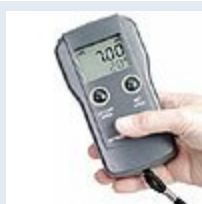
Measure pH of Soil Directly with a Special pH Electrode
