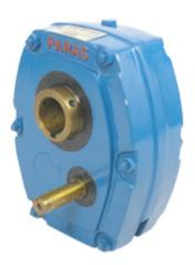
PARAS Shaft Mounted Speed Reducer are compact designed for direct mounting on the drive shaft of the equipment to be driven and also totlly enclosed. This principle assures positive and permanent allignment of the speed reducer and driven machine. And it permits convinient location of the motor, reduces space requirements and layouts problems.
