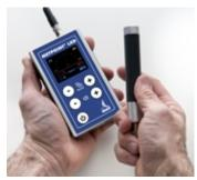
Where compressed air escapes, friction of the gas molecules at the wall of the pipework occurs. This friction produces a high-frequency inaudible ultrasound. The **METPOINT® LKD** detects the ultrasound, transforms it into an audible sound and indicates it optically. The **METPOINT® LKD** operates with extreme reliability. As only those frequencies are detected which occur in the event of leakage, precise location of the leaks is ensured under all types of industrial noise conditions.
