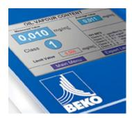
Both METPOINT® OCV systems provide output information about the current measurement value (oil vapour in mg/m³), the ISO 8573 oil class as well as the status of the measuring system and its components. In addition, the status of the measuring cell and the purifier will be displayed visually. You therefore have an overview about the measurement values, oil class, system status at all times and know immediately that your compressed air is correct.
