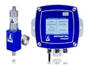
With the stationary dew point measuring device, the data of the continuous measurements are indicated on the display and simultaneously automatically stored in the data logger. An alarm relay is triggered when the adjusted limit value is exceeded. The user will therefore directly receive a message if the process parameters are critical.
