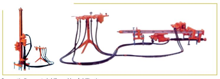
Pneumatically operated drill capable of drilling in both DOWN THE HOLE & JACK HAMMER modes - ideally suitable for drilling lead holes Matching for DIAMOND WIRE CUTTING of decorative MARBLE, GRANITE ROCKS, etc. This machine have Grease filled Rotation & feed Motors, These motors do not require daily oil filling and provide higher penetration rate as compared to conventional oil based Ld4 machine.
