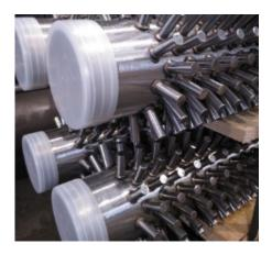
Theses tubes can be manufactured in Straight Lengths of Random Length cut or in Fixed Length. Our Seamless Tubes are manufactured by the Cold Drawn Process (Drawn on Mandrel) to provide the closest dimensional tolerance and smooth Outside and Inside Finish. Further to achieve the desired Mechanical Properties the tubes are Heat Treated (Normalized, Stress Relieved, Annealed, Tempered Etc) as per the Customer/Grade requirement.
