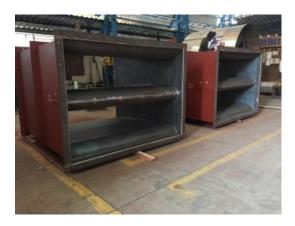
This consists of aerodynamic shaped foils, which offers a very little resistance to the fluid. The typical profile of Aerofoil, offers a smooth passage to the fluid which leads to the lesser pressure drop and thus more efficiency. Aerofoil is supplied with flanged end, thus making the installation in the line, very easy.
