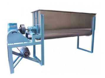
We offer a ribbon blender to our clients for their various industrial needs. The ribbon blender and their sides are manufactured by us from Stainless or Mild steel materials. It comprises of a stainless steel or mild steel centre shaft fitted with specially designed agitator blades for providing the contra flow action. These blenders are equipped with a couple of ribbons. The outer ribbon moves the ingredients into the blender whereas, the inner ribbon constantly circulate the material.
