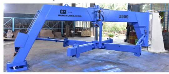
The slewing arms support a spigot former and is mechanically locked. The spigot is formed by the oscillating motions of the hydraulic cylinders located on the arms. Simultaneously, the press head is forced down by the hydraulic cylinder. The spigot length is controlled by the press head. The movement of the arm/s is hydro motored and position- controlled by the PLC.
