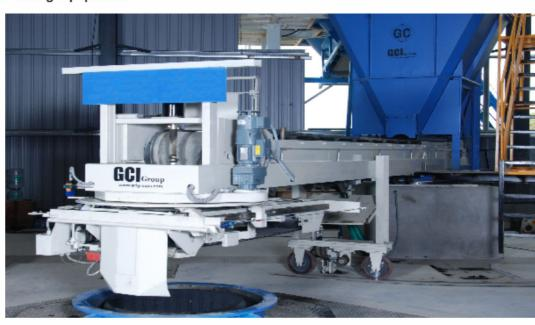
The main and feeder conveyors have vulcanized, heavy-duty conveyor belts. Proximity sensors indicate the position of the feeder conveyor index and pivot.
