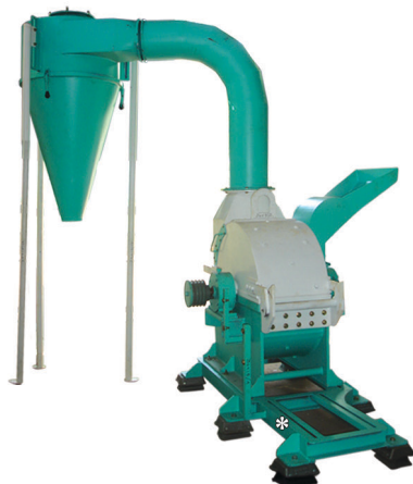
Disintegrator cum blower with cyclone collector
