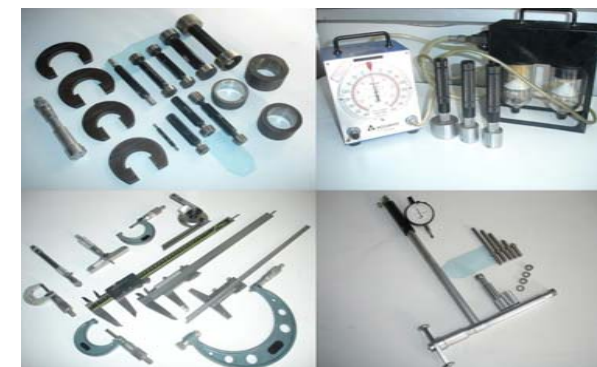
Wide Range of General Purpose Measuring Instruments and Custom Made GO / NOGO Gauges
