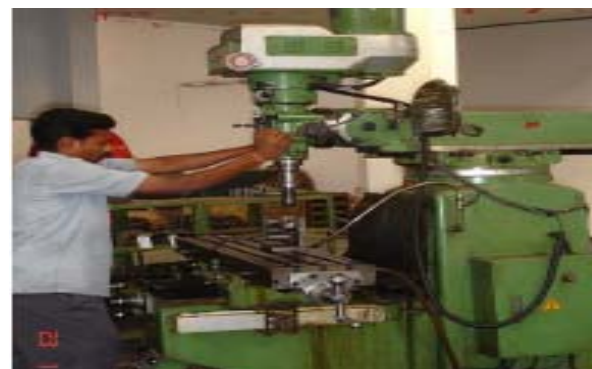
PRECICUT Turret Milling Machine. X-600; Y-400; Z-400. DRO 0.005 mm Resolution
