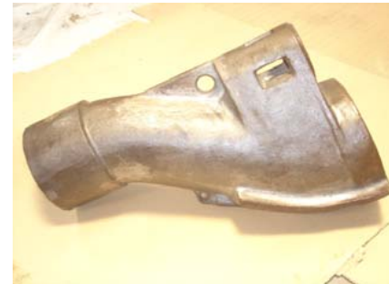
S-Pipe Casting for Concrete Pumping. 1.7218 Steel
