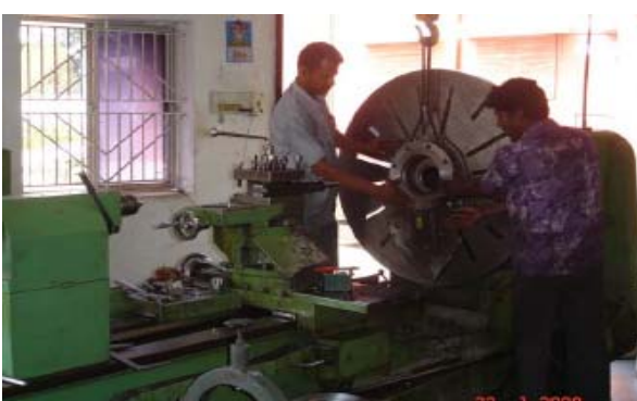
KILOSKAR Conventional Lathe Center Ht 20" x Length 76"
