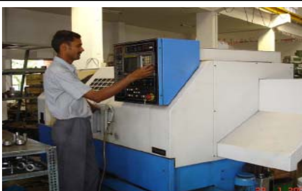
ACE LT020 Turning Center Job Dia 340 mm x Length 600 mm
