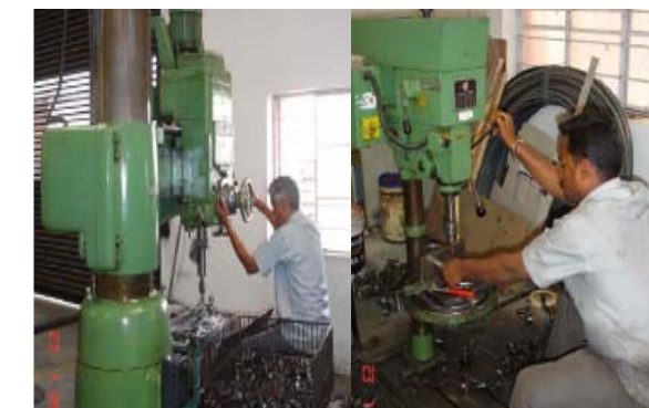
GIRARDS Radial Drilling Machine. Drill Dia 50 mm CKP Pillar Drilling Machine
