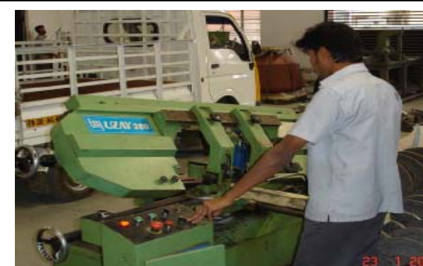
UZAY Band Saw Cutting Machine Dia 10 mm to 180 mm
