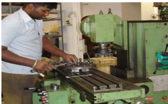
HMT FN 2H Milling Machine X-800; Y-265; Z-400
