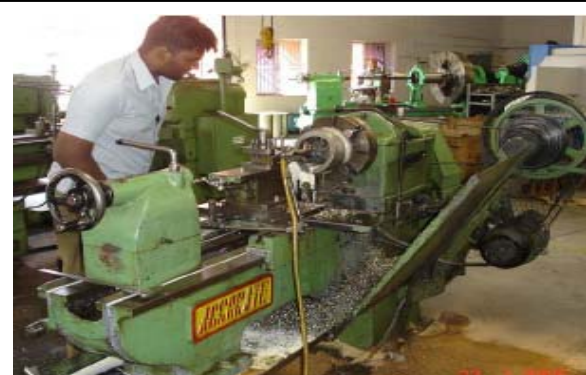
ACCURATE Conventional Lathe Center Ht 10" x Length 40"
