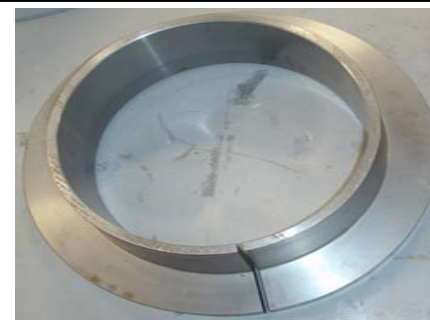
Fully Machined Clamping Ring. GS-52
