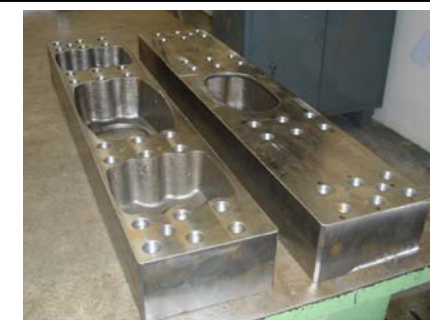
Precision Machined Knotenelement. 1.1138
