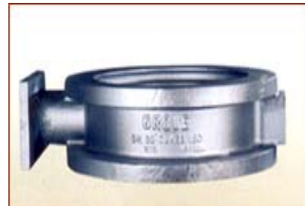
Butterfly Valve Body Castings. 1.0619 Size upto DN 900. Pressure Rating PN10/16
