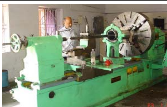
NEW UNITED Conventional Lathe Center Ht 24" x Length 76"
