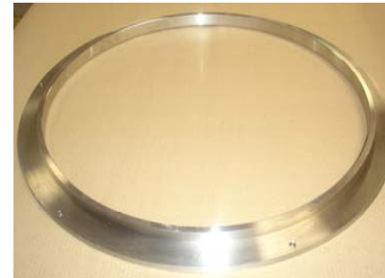
Fully Machined Clamping Ring. 1,4301
