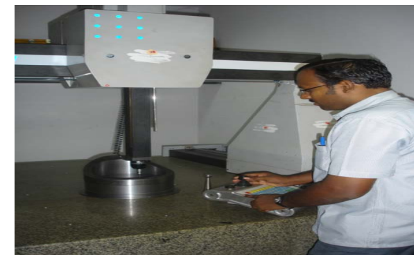
JASH 3-D Coordinate Measuring Machine With State-of-the-art software Range :1000 mm X 700 mm X 500 mm
