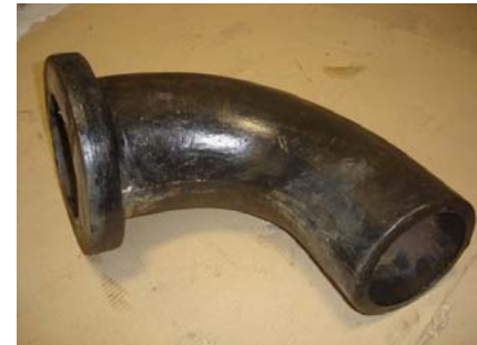
90° Bend Pipe for Concrete Pumping. High Manganese Hadfield Steel 1.0446
