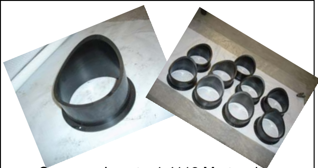
Conveyor Inserts. 1.4112 Martensitic Stainless Steel precise machined and nitrided
