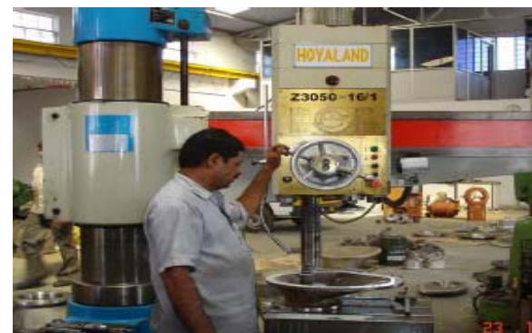
TEAM Radial Drilling Machine Drill Dia 50 mm
