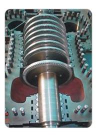
Kessels gets its Rotors machined from a solid alloy forging of a specific metallurgy. These rotors are forged under a strict control on the grain size, the entire manufacturing process and with an adequate reduction ratio. The machining at different stages is done on Conventional and CNC machines to ensure high precision and utmost quality. The trademark of Kessels turbines across different power ranges is the application and use of rotors with a large journal diameter.
