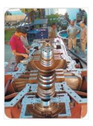
Kessels Casings are rugged and heavy across the entire range, designed with contoured walls and robust flanges to achieve rapid conduction of heat and prevent large temperature gradients. These measures are undertaken to ensure a safe and long operational life.
