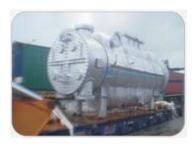
Kessels sources its Condensers from some of the leading manufacturers in India. These Shell and Tube type surface condensers are designed as per best practices and according to the latest HEI and ASME specifications and standards. Rigorous quality practices and the use of adequately sized tubes ensure the condensers supplied with Kessels Turbines have just as long an operating life.
