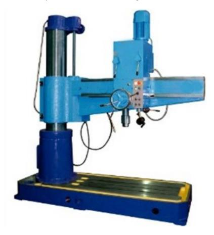
We also provide some optional accessories like heavy duty box table, coolant pump with fittings, machine vice and machine lamp. Our company has come up as one of the prominent Drill Machine Manufacturers and Drilling Machine Exporters. Drill Machine in which the drilling head is mounted to slide along a radial arm which can be rotated, raised, or lowered on a vertical mast to adjust the position of the drill above the workpiece.
