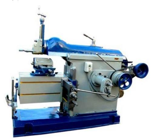
All these Shaper Machines are manufactured using best quality materials and are customized as per the specifications detailed by clients. The work piece mounts on a rigid, box-shaped table in front of the machine. The height of the table can be adjusted to suit this work piece, and the table can traverse sideways underneath the reciprocating tool, which is mounted on the ram. Table motion may be controlled manually, but is usually advanced by automatic feed mechanism acting on the feed screw.
