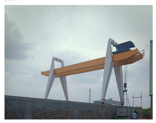
These cranes are appreciated for their attributes like easy installation, lightweight and simple structure. We offer these cranes in single and double main gantry cranes. These Gantry Cranes find high applications in handling and conveying equipment in mills, mines, harbors and enterprise stations. These are generally used outdoors in Engineering Industries, Ship yards, Ports, Granite, Steel Yards, Cement Pipe Industries, Open Yard, Storages places, Container Depots etc.
