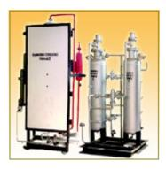
These are Catalytic cracking units in which Ammonia is dissociated to Nitrogen and Hydrogen. Commercial grade liquid ammonia from cylinders or tank is used as feedstock. The Product gas has 75% Hydrogen and 25% Nitrogen. This gas is further purified in a Molecular Sieves unit by removing un-cracked Ammonia and moisture. Purified gas is then used in Heat treatment furnaces like Annealing, Sintering and as Reducing furnace atmosphere.
