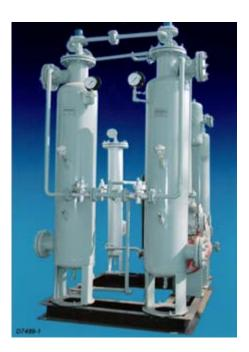
For reducing residual ammonia and to get very dry gas, a Molecular seives based purifier is provided after Ammonia cracking unit. This reduces ammonia down to 1-ppm level and dries gas up to (-) 80 degree celcius dew point.
