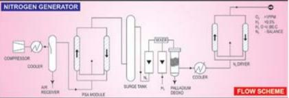
Nitrogen Gas Generators produces Nitrogen gas from atmospheric air by PSA (Pressure Swing Adsorption) Technology. PSA Technique is a simple & reliable process of separation of Nitrogen from compressed atmospheric air by adsorption of oxygen over a bed of Carbon Molecular Sieves (CMS). CMS is an adsorbent having infinite number of small pores. The diameter of the "Bottle Necks" is in the same range as those of the molecules.
