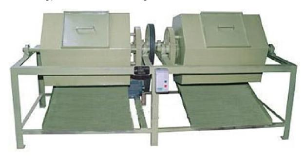
The wire for processes of cutting nails is not so bright and as a result, the nails produced do not have brightness and shinning. Such finished are not acceptable to the buyers thus the nails do require polishing which result in attractive finished products to eliminate this problem. We have manufactured polishing machine.
