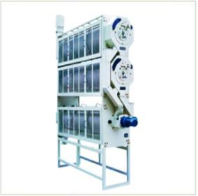
The grains which are longer in length drop out of the indents before they reach the catch trough. The grains which remain in the indents are thrown into the catch trough.
