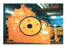
Double Toggle Jaw Crushers use two toggle plates and hence the name. Such crushers do not rub the jaw plates with the material to be crushed and hence lead to lesser production of dust (very small crushed size), higher jaw plate life and lesser power consumption.
