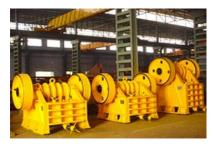
A Single Toggle Jaw Crusher uses only one toggle plate in its mechanism. Two bearings are fit in the swing jaw of this crusher and the other two bearings support the eccentric shaft, which is driven by the drive flywheel. An extra (non-drive) flywheel is provided to lessen the power requirement of the prime mover (motor / engine).
