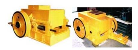
A Double Roll Crusher is based on the principle of feeding the material to be crushed between two manganese steel cast rollers rotating in opposite directions, with their axes parallel to each other.
