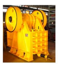
Jaw Crusher, as the name suggests, works on the same principle as the human jaw. It has one stationary jaw (like the upper teeth set) and the other movable (like the lower teeth set) with the material to be crushed (food to be chewed) fed inside the two jaws (mouth) and crushed (chewed) to the desired size and discharged (swallowed) to accommodate fresh input of material (food).
