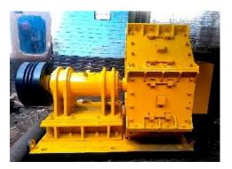
Lakshmi Rotopactor machine is the ultimate weapon against flakiness. It is basically a rotary crusher consisting of an impeller (Rotor) rotating at 1000-1200 r.p.m. inside a steel fabricated body lined with high grade austenitic manganese steel breaker liners. It is used in the secondary or tertiary stage of a stone crushing plant.
