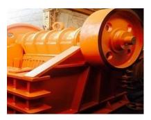
A Jaw crusher uses compressive force for breaking of particles. the mechanical pressure is achieved by the two jaw of the crusher of which one is fixed while the other moves back and forth relative to it, by a cam or pitman mechanism. The inertia required to crush the material is provided by a weighted flywheel that moves a shaft creating an eccentric motion that causes the closing and opening of the gap.
