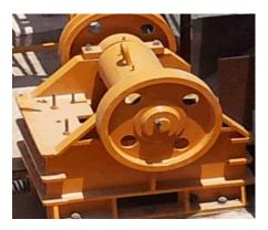
REW Jaw Granulators are heavy duty and have Grease lubrication system. These crusher are designed for long life service with minimum maintenance for hard, tough and abrasive material, including Ferro Alloys. The principal of crusher is on the basis of compression on rock against metal..
