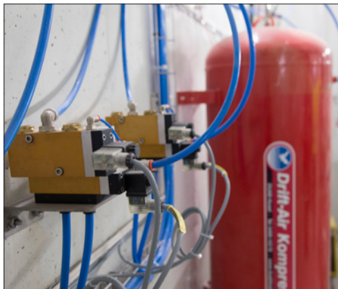
Fail-safe solution with valve package and air accumulator tank
