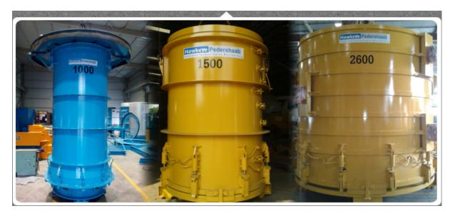
We supply high-quality pallets, headers and set rings, used to form the ever-important joints on the produced precast concrete products.
