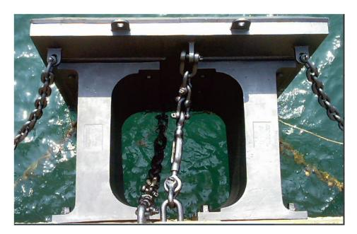
I fender is an energy-efficient buckling type fender. They are used in pairs and can be arranged in various combinations to optimize the overall performance characteristics of the fender system.
