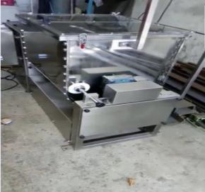
All contact parts of AISI stainless steel 304 material.
