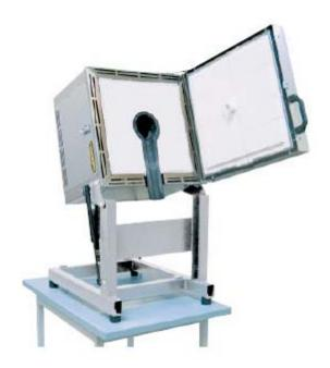
The aluminium melting furnace is made out of mild steel casing and coated with two coats of heat resistance Aluminium paint. The inner chamber will be built with the combination of lightweight refractory bricks & ceramic blanket. Suitable Crucible base will be placed at the bottom of the furnace to take the crucible load along with molten metal.
