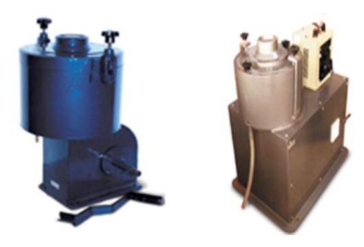
Consists of removable Aluminium rotor bowl of 1500 gm capacity with a cap mounted on vertical Shaft and enclosed in a liquid tight cast housing.
