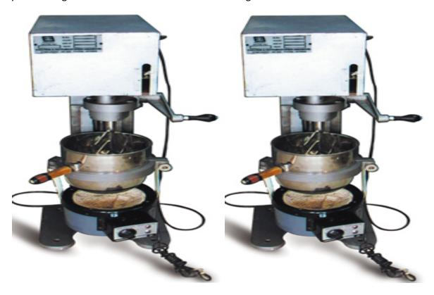
0.5 HP, single phase electric motor connected to epicyclical type stainless steel paddle to impart both planetary and revolving motion for uniform mixing. Mixers have two speeds of 140±5 RPM and 285±10 RPM with planetary motions of approximately 62±5 RPM and 125±10 RPM respectively.
