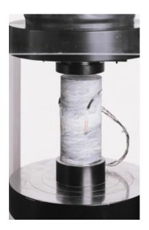
Strain gauges can also be connected, by one or two interfaces 82-P0398, to a suitable data logger as, for example, our model 82-P9008 when the load application on the specimen is performed with Automatic compression testers as, for example the AUTOMAX and PILOT models. In this case, one of the channels of the Datalog 82-P9008 should be used for the load signal coming from an additional pressure transducer with selecting valve fitted to the compression tester.
