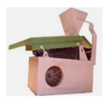
De-stoners" or grain separators are highly functional destoner machinery and have found several applications such as separating heavier materials like stones, glass, metal etc. from food grains and other dry granular material
