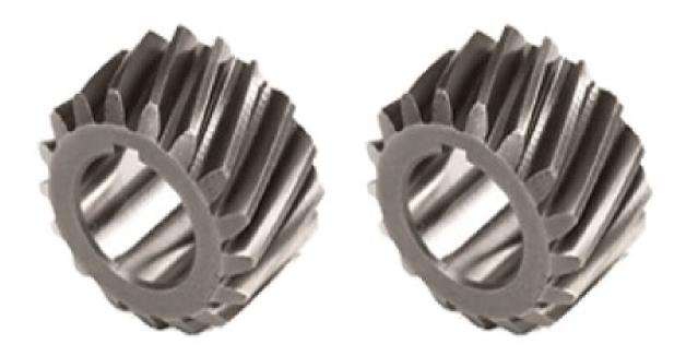
Since the gear is curved, this angling makes the tooth shape a segment of a helix. A pair of helical gears have the same helix angle but the helix hand is the opposite. Helical gears can be meshed in parallel or crossed orientations. The former refers to when the shafts are parallel to each other; this is the most common orientation.
