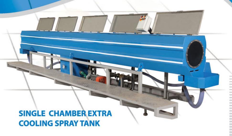
Single Chamber Extra Cooling spray tank is used for an additional cooling of pipes for higher output pipe extrusion line
