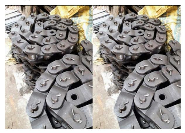
Each component is made from high-quality steels and then specially heat-treated to provide maximum performance and long wear life. Joint parts are hardened to provide greater strength and wear resistance. Sidebars are hardened to achieve ultra-high strength throughout.
